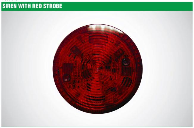
Conventional wall mount sounder with red strobe, designed for installing in conventional fire alarm systems. Supports 32 different tone types and two sound levels, controlled by jumpers. The device is equipped with two additional separate inputs for Alarm and Evacuation events. The tone sounds of the inputs are different for easy recognition from the users on the protected site. The Evacuation event is with the highest priority. Certified according to standard EN54, part 3.
